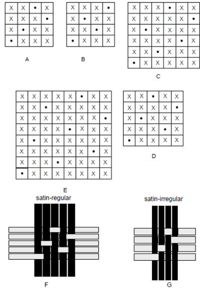
Fig: Example of Satin regular and irregular weave structure
